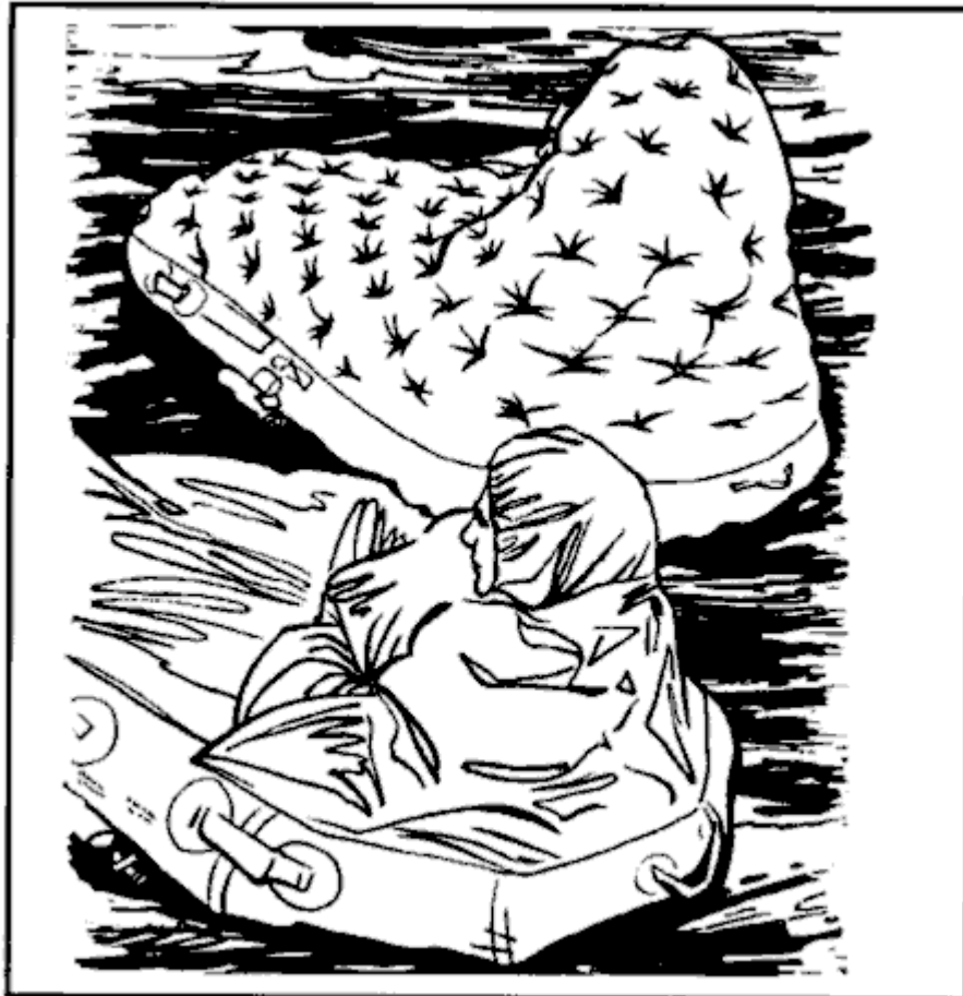
Figure 16-11. One-man raft with spray shield inflated.
